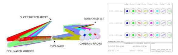
Left: Zemax optical layout of the IFU. Right: Spot diagram at diffraction limit of the IFU, Each column represents a piece of the output slit.
