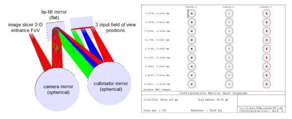
The ZEMAX optical layout of the tip-tilt FoV scanning system presents an optical quality limited by diffraction. This FoV scanning system and the image slicer will be coupled and different geometrical distributions are being considered to fix the systems to the available space at GREGOR. Commercial elements are being considered for the tip-tilt scanning system.
